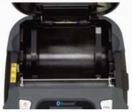
40 - 80mm variable media width support for 0.053 -0.12 mm receipts & up to 0.15mm traditional & liner-free MAXStick labels
